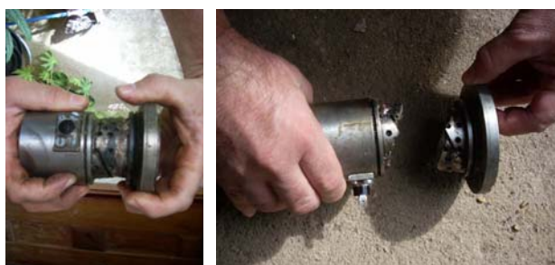
Images of the broken press head
